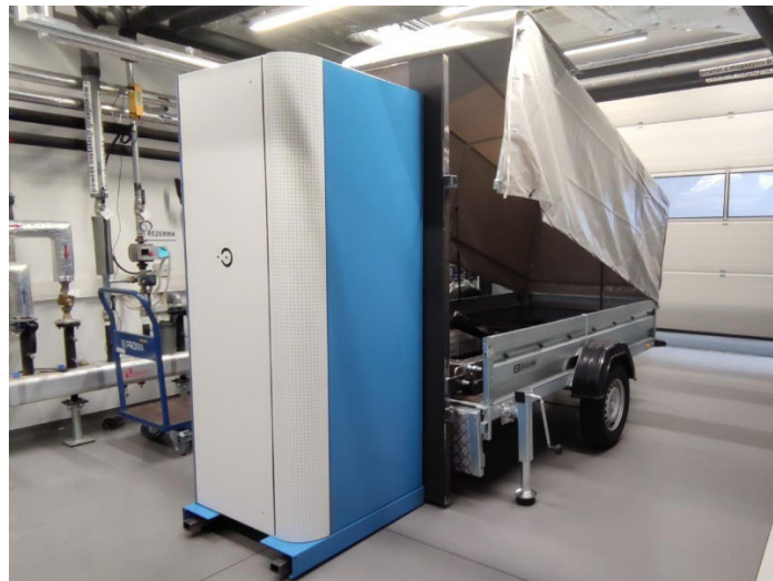
Figure 42 Mobile energy storage: all-in-one cabinet and dedicated transport trailer.
