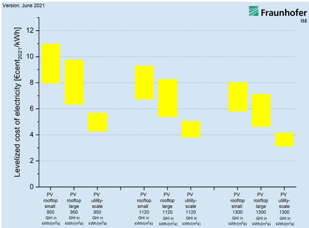
Figure 6. LCOE of PV systems in Germany based on system type and solar irradiation (GHI in kWh/(m²a)) in 2021, [17]
