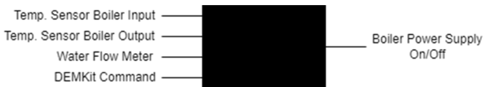
Figure 13. Black box diagram of Saxion E-boiler control system
